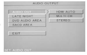
**Note:** The AUDIO OUT setting does not affect the digital coaxial and optical outputs. The format of the digital signal at the coaxial and optical output jacks is determined solely by the DVD being played and the settings in the DVD disc setup menu.
